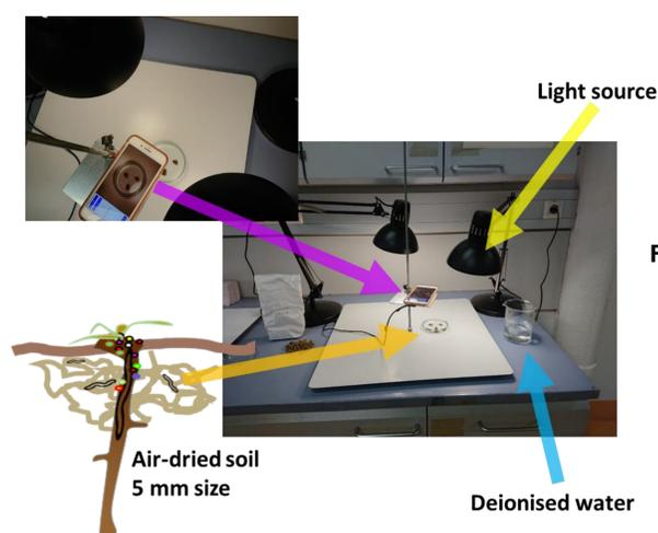
**Figure 2** Laboratory set-up of SLAKES analysis.
