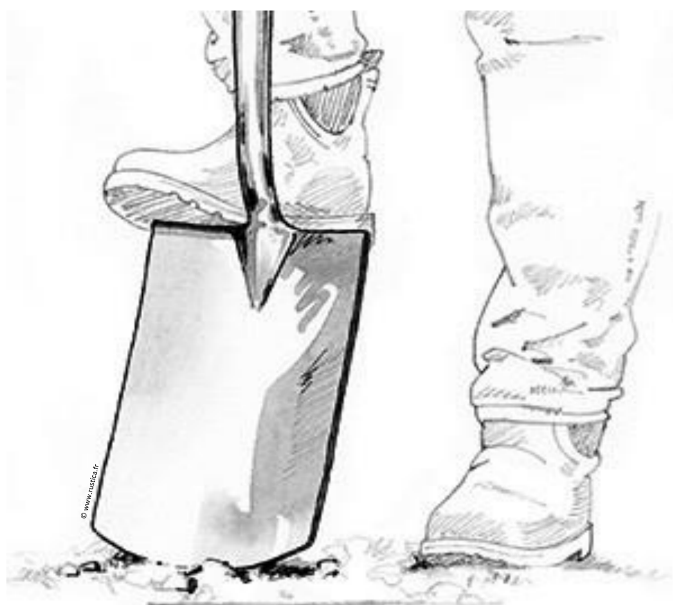
Protocol ISO 23611-1:2018 « Spade test » from EcoBioSoil (Rennes) Chemical extraction and/or hand sorting
